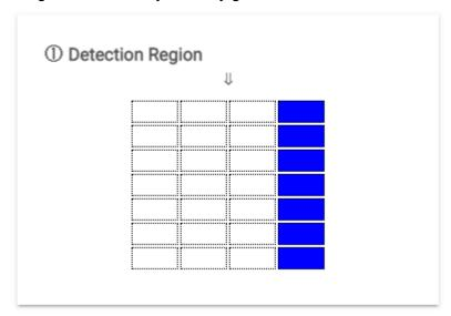
A bitmask that represents the rows of the grid can be sent to the specific region cluster to activate it. For example, in the grid above the data of [1,1,1,1,1,1] would be sent to the cluster.
