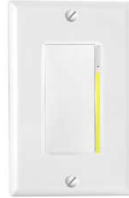
YELLOW Poor Range of ZigBee Signal
