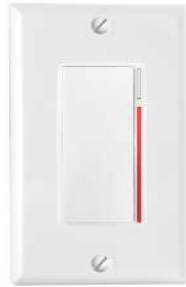
RED Not in Range of ZigBee Signal
